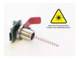
**Figure 20.4.:** Light source module removed from the Cypher AFM. During the removal process it is possible to tamper with safety overrides in such a way that collimated light shines out of the module. As a safety precaution, never look directly into the module while its power cable is attached (power cable not shown in this image).
