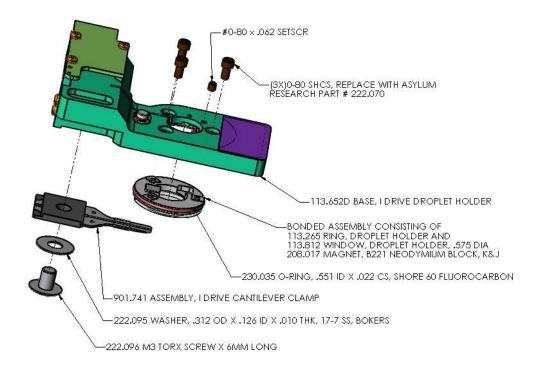
Figure 7.2.: Droplet Cantilever Holder Assembly exploded view
