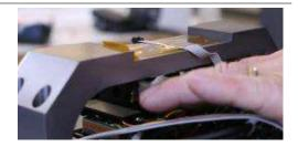
Put lens tissue and Kapton tape over the hot mirror and wrap tape around to cover the side port hole.
