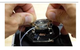
Loosen fittings of gas in/out lines: In this step, you will remove the gas in/out lines. Notice that the gas lines are sealed by a small O-ring which may or may not come out when you pull out the gas lines.
