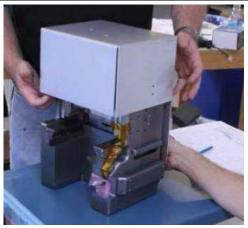
1-2 screws need to go in either side using a 1/8" Hex Wrench L-key (part#290.119). (SCREW INFO: 10-32 x ¼ or ½ BHCS SS depending on which guard you have)
