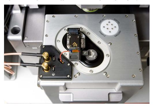
Figure 3.2.: Detailed view of the high voltage option.
