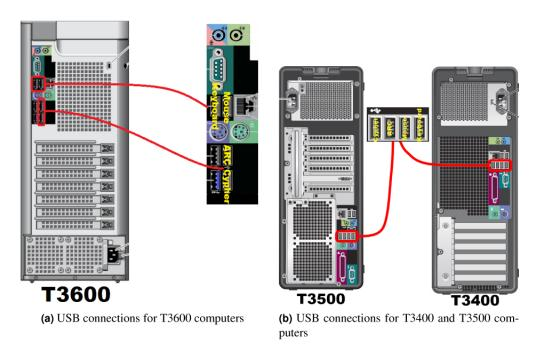
**Figure 22.1.:** If you have a Dell T3600, T3500, or T3400 workstation, please see the following graphics for the best way to set up the USB connections. Connecting in this manner will insure that the Cypher and the ARC will not compete with other USB devices for bandwidth.
