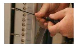
Remove the piece of foam from inside the chassis nearest the backpack screws you just loosened.
