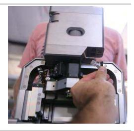
Remove the FireWire cable from the bottom side of the view module (black cable-like USB).
