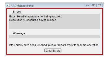
This error is caused by the Feedback Sensor (Head Sensor) not being read. The possible causes can be:
