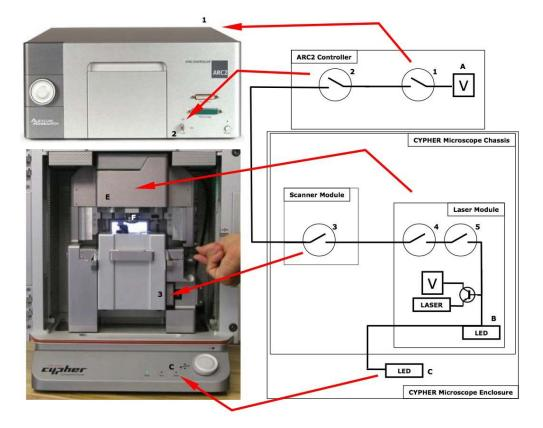
**Figure 20.5.:** Cypher and ARC2 laser safety interlock system. (A) Laser Voltage Source. (1) Back panel remote interlock connector, or Light Source Remote Jack. (2) Front panel laser power key switch. (3) Scanner interlock. (4,5) Laser module dual magnetic switch interlock. (B) Laser Module LED. (C) Cypher enclosure laser LED. (E) Optical system cover. (F) Objective Lens. Not shown is an additional software controlled laser power switch.
