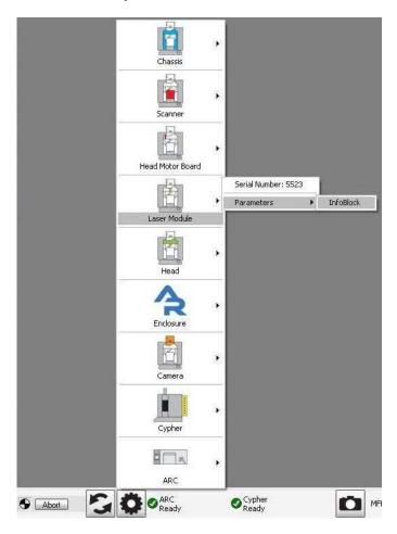
**Figure 18.1.:** To open the Light Tube (Laser Module) infoblock, click on the "gear" icon at the bottom of the screen, then mouse up to the Laser Module and over to the infoblock. Then release the mouse button.
