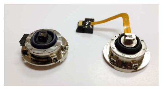
**Figure 13.7.:** Ambient stage / fluid cell body combination on the left. Heater stage / Gas cell body combination on the right.
