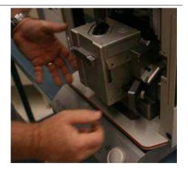
Unscrew the scanner connector cable on the right side of scanner, and loosen the knob to release it.
