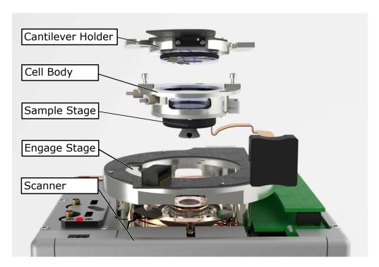
Figure 10.1.: Cypher Environmental Scanner Basic Parts
