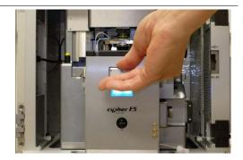
**6.** Now go and clear out a place to set the scanner down once you remove it. We recommend you first place the scanner right in front of the AFM system, and then grip the scanner again to move it elsewhere. If the scanner is dropped it might become irreparably damaged.
