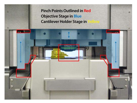
**Figure 20.1.:** Areas to avoid in particular when motors are driving the objective lens or cantilever holder. Tinted parts can move as shown by the arrows.
