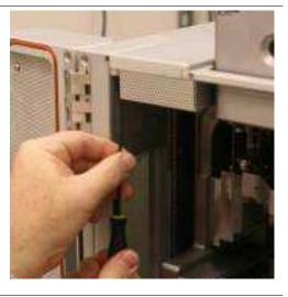
Replace all 4 screws from the back edge of the enclosure top plate. They are visible above the backpack. (SCREW INFO: 8-32 x ½ BHCS SS)
