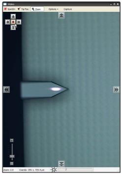
**(b)** The focus offset is centered and the optical image is confocal with the focused laser spot.
