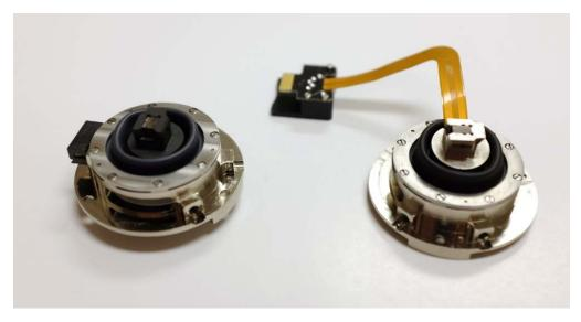
**Figure 13.6.:** Ambient stage / fluid cell body combination on the left. Heater stage / gas cell body combination on the right.
