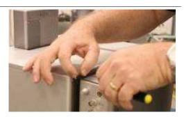
e) Unscrew 2 screws in the right door on the bottom and set aside (note: there may only be 1 screw) - (SCREW INFO: 8-32 x ½ BHCS SS).
