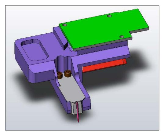
Figure 9.1.: Cypher STM tip holder. Note the probe tip sticking from the small tube.
