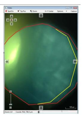
**4.** One way to confirm this is to note the focus position distance located just below the arrow buttons. Raise the objective back up to focus on the field diaphragm and note how much the focus distance has changed. Typically, the sample focus distance is about 30μm below the focus distance of the field diaphragm.
