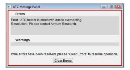
This error is the result of the ATC overheating internally which has caused one of the two thermal switches to trip. A high pitched audible alarm will also sound. The possible reasons for this error to happen can be:
