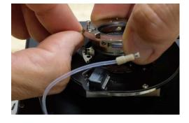
**5.** Check the gas lines to see if small O=rings are stuck to the end. Usually the rings will stay inside the cell, but in case they are stuck to the gas lines, please unstick them and place aside.
