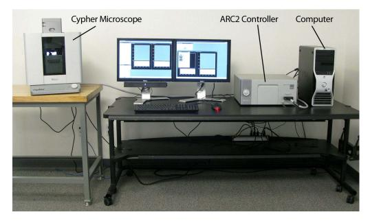
**Figure 1.1.:** Ideally the Cypher SPM is set up as shown, with the controller and computer on one table and the microscope on its own table. The air temperature controller (ATC) is not shown here. Please see Chapter 19 on page 203 for more information.
