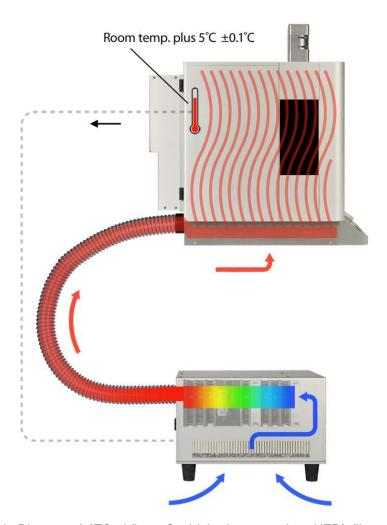
**Figure 19.1.:** Basic Diagram of ATC airflow. Cool lab air enters via a HEPA filter at the bottom of the Cypher ATC and then passes through fans and heater coils and travels via corrugated hose to the Cypher enclosure. Temperature signals travel from the Cypher back to the ATC (dotted line). Air exits the Cypher from the bottom rear.
