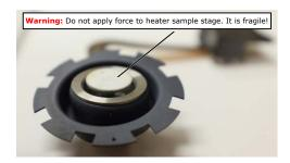
**Note** Although it is not required, lowering the cantilever holder stage fully (with the cantilever holder removed!), will make it easier to exchange samples without touching the heater stage.
