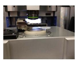
**5.** Secure the droplet holder to the engage pillar by tightening the dovetail clamp. Remember to only hold the driver tool with your fingertips and gently tighten the screw.
