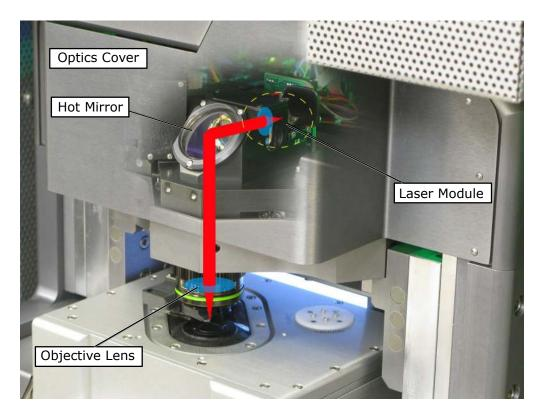
**Figure 20.3.:** Simplified laser path. Removing the optics cover exposes the hot mirror and laser module. The non-visible laser light originates in the laser module and comes out as a collimated beam. The collimated beam is reflected off of the hot mirror and into the objective lens, which focuses it onto the cantilever. During normal operation the only place a person can be exposed to the light is where the light exits the objective.
