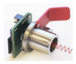
The following instructions describe exchanging light tube assembly in the Cypher AFM. The light tube can be exchanged without disassembly through the front of the instrument with a little familiarity of the process. For the reason of clarity the instructions describe exchanging the light tube by disassembling the enclosure followed by the process done through the front of the instrument.
