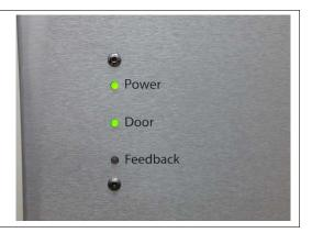
Normal Operation, ATC ON, and controlling temperature. The ATC is on, The door is closed and the ATC Feedback is ON.
