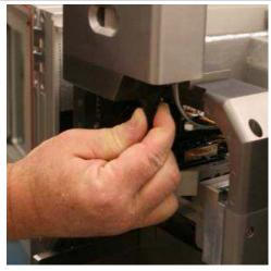
Unscrew and remove 2 screws from the top bridge of the view module using the 3/16" Ball End Allen Wrench L-Key.
