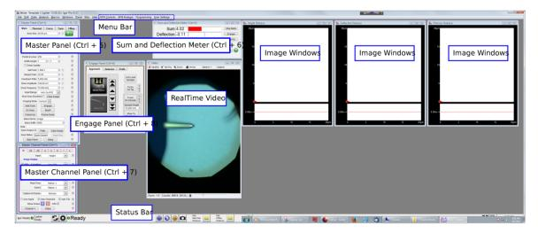
**Figure 1.3.:** Typical start-up screen for the Asylum Research SPM Software. A few image panels have been cut off in this figure. Usually they are found across the second monitor of your system.
