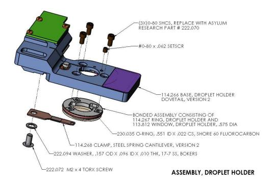
Figure 6.3.: Droplet Cantilever Holder Assembly Overview
