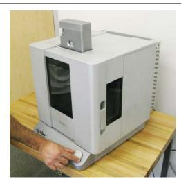
**3.** Turn the ARC2 controller power off. This will shut off most of the Cypher's power. It is not necessary to disconnect the motor power supply when exchanging the light tube assembly.
