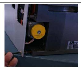
Now turn the nut back toward the screw head and tighten it with pliers (Pliers not provided with system) – one on each side. (SCREW INFO: 10-32 x1 ½ or1 ¾ BHCS SS depending on which guard you have & 2 10-32 Kepnuts.)
