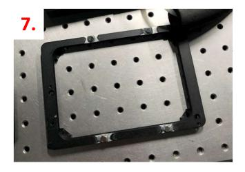
Place the holder into the stage of the microscope, then put the incubation chamber in the holder.
