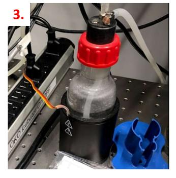
Make sure the humidity module is filled with water. The air will bubble through.
