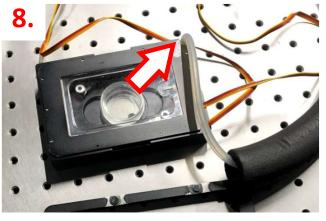
Connect the insulated tubing from the humidity module.
