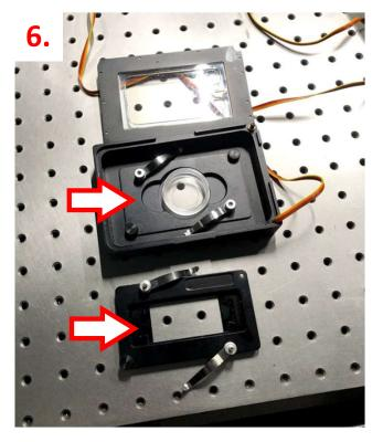
Mount to correct inset for slides or dishes into the incubation chamber.
