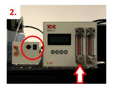
Turn the air pump on.
