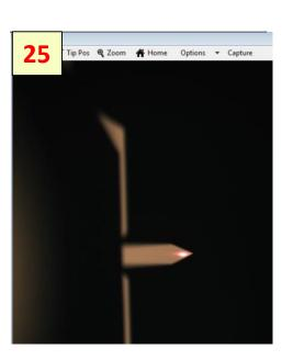
You will now be prompted to focus on your tip. Use the engage panel to move the focus up or down with the arrows. The single arrow produces small movements and the double-arrows produce larger ones. When you are satisfied with the focus, press the "tip is focused" button on the GetStarted Panel.
