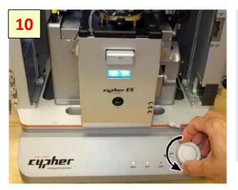
To load or unload a sample, you will need to lower the coarse engage stage so that you can access the sample stage.
