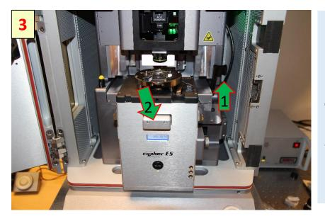
1.Unlock scanner: Lift the lever to the right of the scanner.2.Pull the scanner forward:
