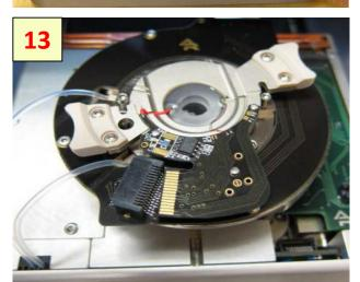
**Place cantilever holder:** The cantilever holder should sit level and be rotationally aligned so that the cantilever holder board is almost touching its mating connector.
